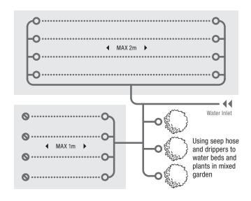
KIT REQUIRED: SOL-C24L, 12 Dripper Ext Kit, 12m Seephose Spare Capacity: 9 drippers
