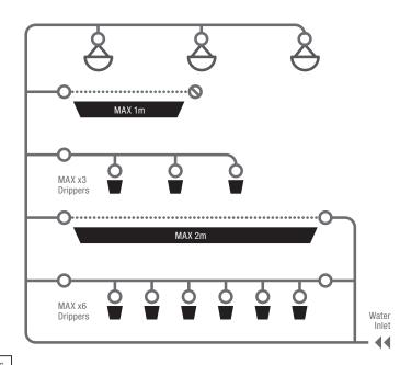
KIT REQUIRED: SOL-C24L, 12 Dripper Ext kit, 12m Seep Hose Spare capacity: 6 Drippers
